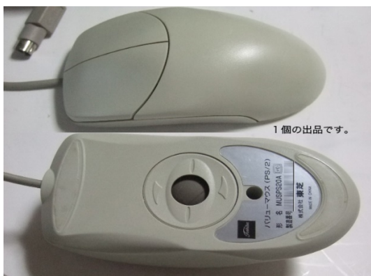
Fig : ball-type mouse
